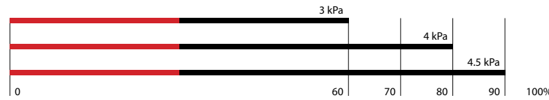
CYCLIC TESTING AT 5.0 kPa WITH 2 NAILS BATTEN/RAFTER FIXING AND 4 NAILS PER TILE SECTION
